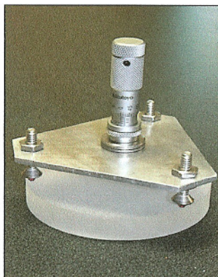
3.5" spherometer used to measure radius of curvature
